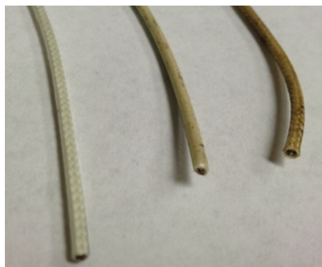
Figure 3.2 Photo of a selection of the 17 wire specimens. From left to right: wires I, M and A. Note the severe discoloration in wire A, which was found to have been highly degraded.
